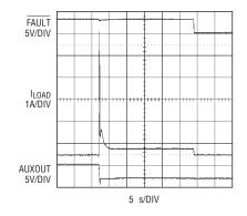
Figure 6. Fast acting current limit isolates short-circuit fault on 3.3V auxiliary output
