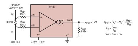
Figure 2. Typical LT6105 connection. Sense resistor is  $20m\Omega$  and gain is 50, so the transfer function is  $V_{OUT}/I_{LOAD}$  = 1V/A. Note the wide input source.
