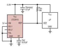
Figure 4. A 1V, -15% tolerance supply monitor with 90ms timeout
