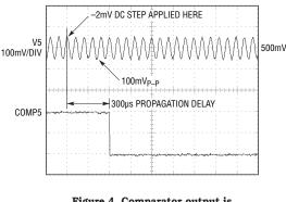
Figure 4. Comparator output is resistant to noisy input voltage
