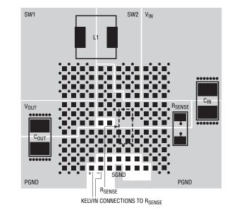
Figure 11. Kelvin connection used to sense current.
