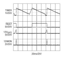
Figure 7. Auto-retry with 0.5% duty cycle during 12V output short
