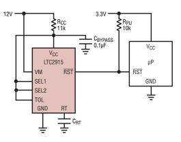
Figure 1. A 12V supply monitored from 12V, utilizing internal shunt regulator with 3.3V logic out
