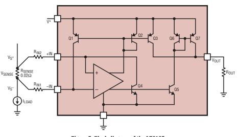
Figure 5. Block diagram of the LT6105
