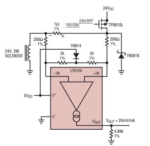
Figure 8. Similar circuit to Figure 6 but with solenoid grounded, so freewheeling forces inputs negative. Providing resistive pullups keeps amplifier inputs from falling outside of their accurate input range.
