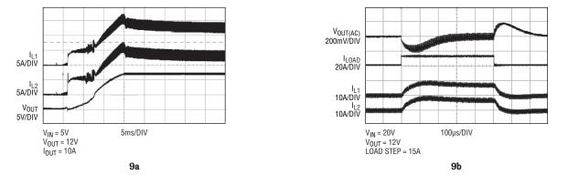
Figure 9. Inductor current waveforms at start-up and load transient with two LTM4607s in parallel
