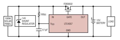
Figure 2. Solar panel charging 12V battery through ideal diode to prevent back feeding
