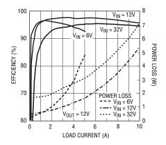
Figure 6. Efficiency and power loss for the LTM4607 at different input voltages
