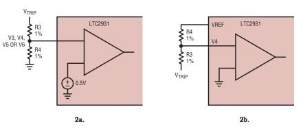
Figure 2. Using a resistive divider to set the voltage trip point
