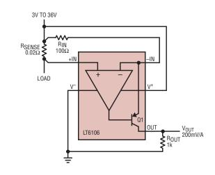
Figure 1. Typical current sense application using the LT6106. Sense resistor is  $20m\Omega$  and gain is 10, so transfer function is  $V_{OUT}/I_{LOAD} = 0.2V/A$ .
