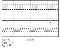
Figure 4. Boost mode waveforms
