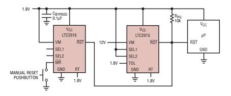
Figure 7. Dual supply monitor (1.8V and 12V) with manual reset and 200ms Reset timeout
