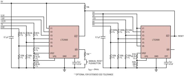
Figure 6. Wired-OR system reset
