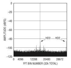
Figure 3. An FFT of the LTM9001 at 160MHz input frequency with the randomizer on
