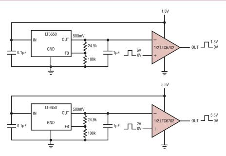
Figure 3. Level translation without the need of an additional supply or pull-up resistor
