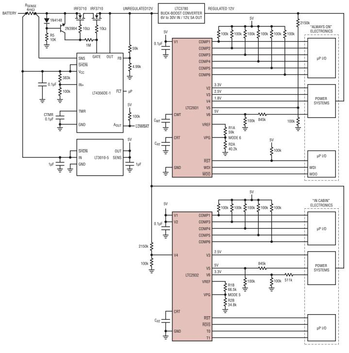
Figure 10. The LTC2931 and LTC2932 in an automotive application
