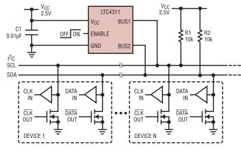
Figure 4. Typical LTC4311 application with low current shutdown
