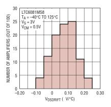
Figure 1.  $V_{OS}$  drift histogram of LTC6081
