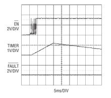
Figure 2. TIMER blanking time prevents false fault reset from  $\overline{\rm EN}$  pin contact bounces.
