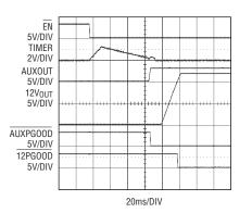
Figure 3. Normal power-up sequence with  $C_{L1}$  = 2200µF and  $C_{L2}$  = 150µF after a debounce timing cycle
