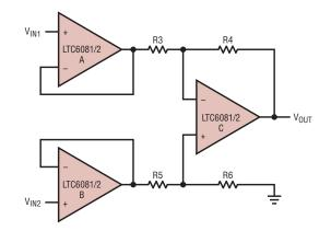
Figure 3. Instrumentation amplifier with unity gain buffers
