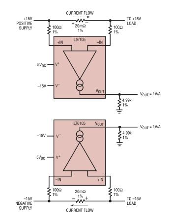
Figure 9. The LT6105 can monitor the current of either positive or negative supplies, without a schematic change. Just ensure that the current flow is in the correct direction.
