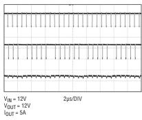
Figure 5. Transition mode waveforms
