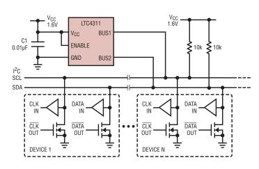
Figure 1. Typical LTC4311 low voltage application circuit
