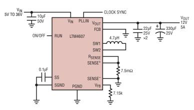
Figure 1. Remarkable simplicity in the face of an otherwise daunting task. Only a few components are required to provide an efficient 12V, 5A output from a 5V-to-36V input.
