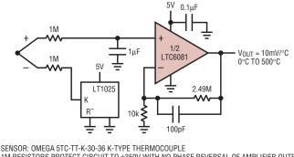
SENSON: UMEGA 51C-11-K-30-36 K-1YPE I HERMOCOUPLE 1M RESISTORS PROTECT CIRCUIT TO  $\pm$ 350V WITH NO PHASE REVERSAL OF AMPLIFIER OUTPUT 1pA MAX I<sub>BIAS</sub> TRANSLATES TO 0.05°C ERROR 90µV V<sub>OS</sub>  $\rightarrow$  2°C OFFSET
