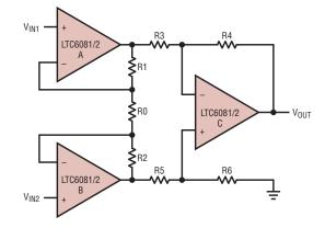
Figure 2. Typical three op amp structure of instrumentation amplifier
