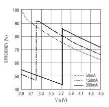
Figure 1. Efficiency vs V<sub>IN</sub> for various LED currents
