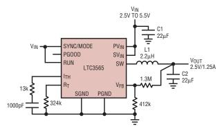
Figure 2. Battery to 1.2V at 1.2A application of the LTC3565
