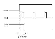
Figure 2. LT3518 timing diagram
