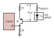
Figure 11. Open LED protection setup for buck configuration
