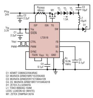
Figure 9. Buck mode 1.5A LED driver
