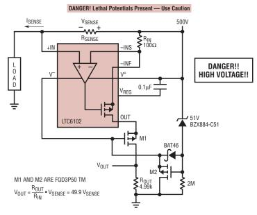
Figure 4. Simple 500V current monitor
