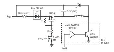
Figure 3. External PMOS disconnect switch driver for a conventional LED driver
