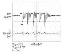
Figure 6. Operating waveforms
