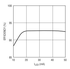
Figure 4. Efficiency of the 160-LED driver shown in Figure 3 is over 92%.
