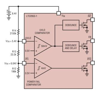
Figure 5. De-glitched UVLO comparator monitors battery stack
