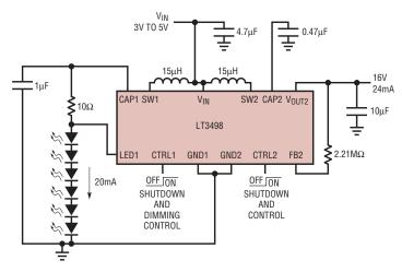
Figure 1. Li-Ion to six white LEDs and an OLED display
