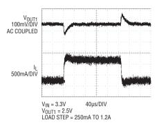
Figure 5. Load step response
