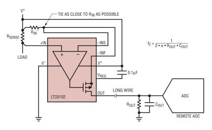
Figure 6. Remote current sense with simple noise filter
