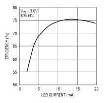
Figure 2. Efficiency of the circuit in Figure 1
