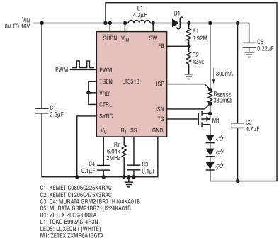
Figure 7. Buck-boost LED driver for automotive applications
