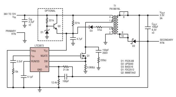
Figure 1. A nonisolated flyback converter
