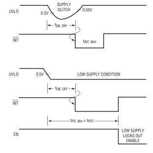
Figure 6. Low supply initiates system power down and locks out enable
