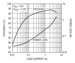
Figure 4. Efficiency and power loss for Figure 3, Channel 1.
