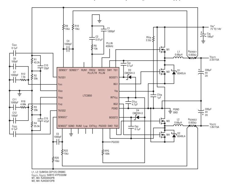
$^{\star}$  FOR  $V_{\mbox{\footnotesize{IN}}}$  = 5V  $\pm$  0.5V, TIE  $V_{\mbox{\footnotesize{IN}}}$  AND INTV $_{\mbox{\footnotesize{CC}}}$  PINS TOGETHER.
