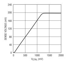
Figure 3. LED sense voltage versus CTRL pin voltage
