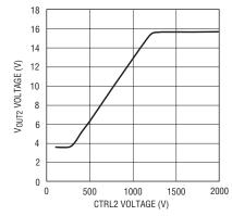
Figure 5. V<sub>OUT2</sub> voltage vs CTRL2 pin voltage
