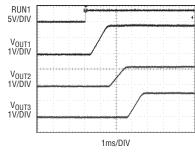
Figure 3. PGOOD pins allow simple power sequencing. Soft-start reduces inrush currents and prevents output voltage overshoot.
