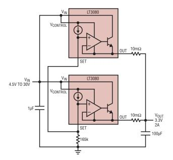
Figure 6. Paralleling of two regulators. Need more current? Add more regulators. Current sharing is assured by the  $10 m\Omega$  PC board traces, which act as ballast resistors.
