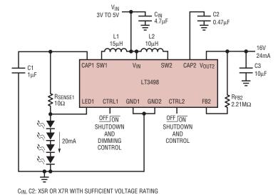
Figure 9. Li-Ion to four white LEDs and an OLED display
