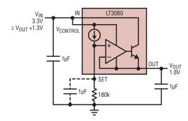
Figure 4. Basic hookup for the LT3080 regulator. The IN and  $V_{CONTROL}$  pins are tied together and a single resistor sets the output voltage. A 1µF output capacitor ensures stability. If the adjustment resistor is adjusted to zero, the output is zero.
