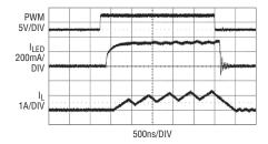
Figure 8. 3000:1 PWM dimming waveform of application circuit of Figure 7 at 120Hz PWM frequency and  $V_{\rm IN}$  = 12V.
