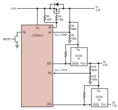
Figure 7. Pushbutton controlled supply sequencing
