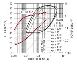
Figure 5. Efficiency in normal mode and Burst Mode operation
