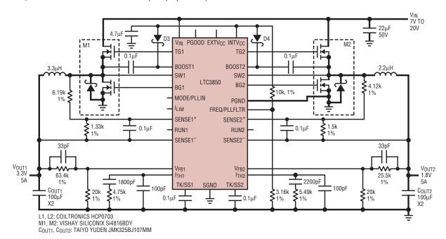
Figure 3. Schematic for a 2-channel, 5A/500kHz regulator with DCR sensing.
