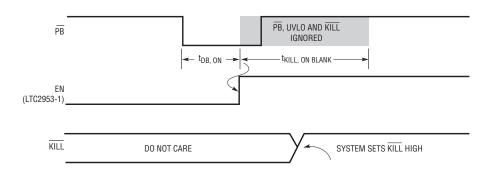
Figure 2. Timing diagram shows a pushbutton-controlled system power on.
