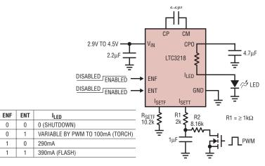
Figure 3. LED driver uses pulse-width modulation to implement dimming and brightness control
