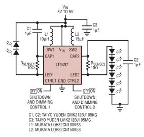
Figure 8. Li-Ion to a 2-LED and 6-LED Display
