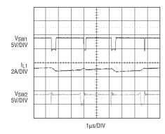
Figure 4. Input-side and output-side switch waveforms along with inductor current for buck-boost mode (3.8 $V_{\rm IN}$ )
