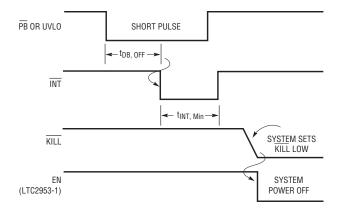
Figure 3. Timing diagram for normal power off sequence
