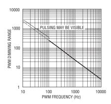
Figure 7. Dimming Ratio Range vs Frequency
