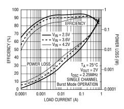
Figure 6. Burst Mode operation maintains high efficiency at low load currents.
