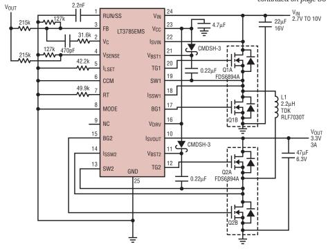
Figure 1. Schematic of buck-boost converter using LTC3785 to provide 3.3V at 3A out from a 2.7V-10V source
