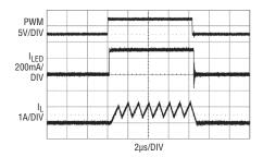
Figure 6. PWM dimming waveform for Figure 5 at 120Hz PWM frequency and  $V_{\rm IN}$  = 10V
