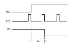
Figure 1. Regular LED driver timing diagram
