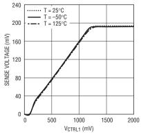
Figure 4. LED sense voltage vs CTRL1 pin voltage
