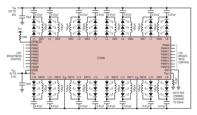
Figure 1. A 16-channel LED driver. The 15V-45V input is used to drive three white LEDs per channel with 5000:1 PWM dimming.
