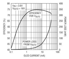
Figure 3. Efficiency of the OLED Driver in Figure 1
