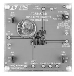
Figure 1. The LTC3545 is a compact solution to the problem of multiple voltage supplies.
