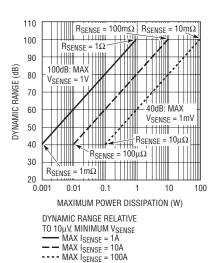
Figure 2. Dynamic range vs maximum power dissipation in R<sub>SENSE</sub>
