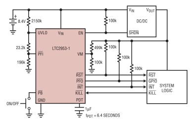
Figure 1. A complete pushbutton and voltage monitoring system is easy to set up with the LTC2953-1.
