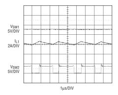
Figure 3. Input-side and output-side switch waveforms along with inductor current for boost mode (2.7 $V_{\rm IN}$ )
