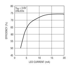
Figure 9. Efficiency of the circuit in Figure 8
