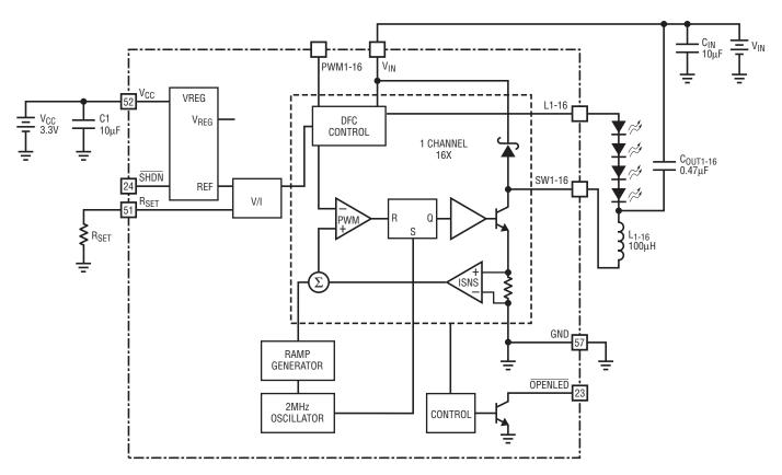
Figure 5. Block diagram for the LT3595
