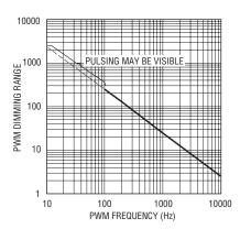
Figure 8. LED dimming range vs PWM dimming frequency
