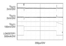
Figure 4. Channel-to-channel transient crosstalk is negligible.
