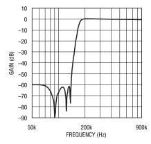
Figure 10. Frequency response of Figure 9's circuit
