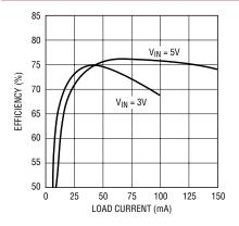
Figure 10. 5V to -5V inverting converter efficiency reaches 76%.
