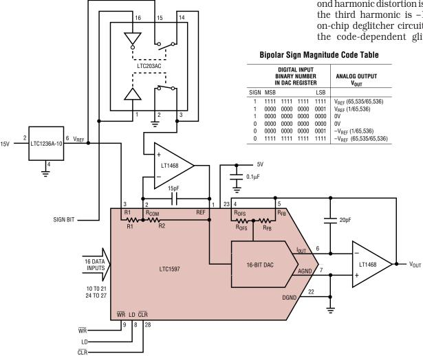
Figure 8. This 17-bit sign-magnitude DAC uses the LTC1597 in its unipolar mode with the reference bit inverted ( $-V_{REF}$ ) for the output range 0V to  $V_{REF}$ . When the sign bit changes, the analog switch changes the reference input polarity to noninverting ( $V_{REF}$ ) for the output range 0V to  $-V_{REF}$ . The resulting circuit produces an impressive bipolar zero error of 140 $\mu$ V (0.92LSB) max at room temperature—less than 1LSB at 17 bits.
