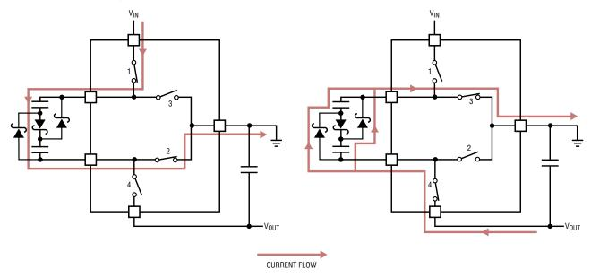
Figure 4. Adding three diodes to a switched capacitor inverter doubles the current between the input and the output.
