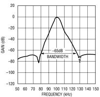
Figure 6. Measured amplitude response of Figure 5's filter
