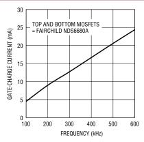
Figure 4. MOSFET gate-charge current vs frequency
