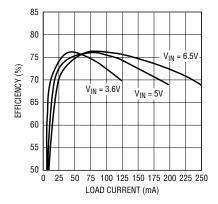
Figure 7. Efficiency of Figure 6's SEPIC reaches 77%.
