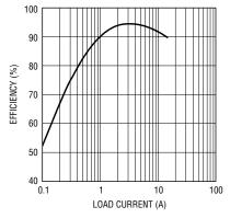
Figure 2. Efficiency of Figure 1's circuit
