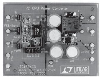
Figure 1. LTC1736 evaluation circuit: a complete 5V-24V to 0.9V-2V/12A converter in  $2.15 \mathrm{in}^2$  of PC board space
