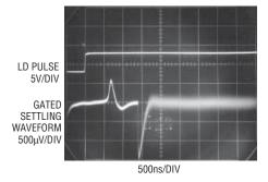
Figure 4. When used with the LT1468 and a 20pF feedback capacitor (see Figure 3), the LTC1597 can settle in an amazing  $1.7\mu s$  to within 0.0015%. The top trace shows the LD pulse; the bottom trace shows the gated settling waveform settling to 1LSB in  $1.7\mu s$ .
