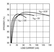
Figure 17. 4-cell to -10V converter efficiency
