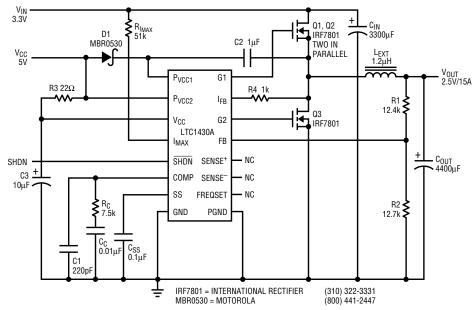
Figure 3. 3.3V to 2.5V/15A converter using a 5V auxiliary supply and the LTC1430A
