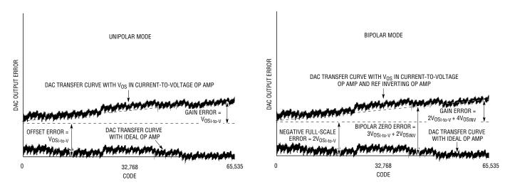
Figure 10. The effect of op amp offset on the LTC1597 gain and offset errors in unipolar mode (left) and bipolar mode (right); op amp offset has virtually no effect on DAC linearity; it merely shifts the end points.
