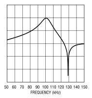
Figure 4. Cascading two 4th order bandpass sections to realize the filter of Figure 3.
