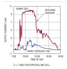
Figure 7. Charging profiles for two square inch photovoltaic cell
