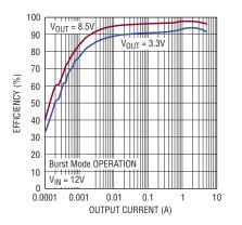
Figure 4. Efficiency in Burst Mode operation for the two outputs. Due to its low  $I_{Q}$  in Burst Mode operation, the LTC3890 maintains high efficiency and low power loss operation down to very light loads.
