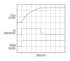
Figure 4. High density capacitor charger
