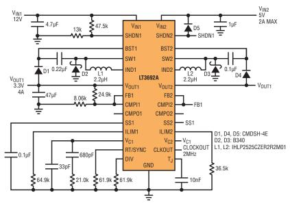
Figure 18. Dual input single 3.3V output converter
