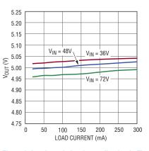
Figure 3. Load regulation for application in Figure 2
