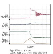
Figure 4. Overvoltage protection waveforms when 20V adapter is plugged into 5V system
