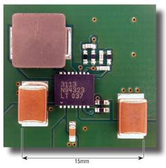
Figure 1. A typical application occupies 154mm<sup>2</sup>
