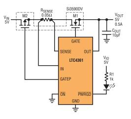
Figure 1. A 5V system protected from ±24V power supplies and overcurrent
