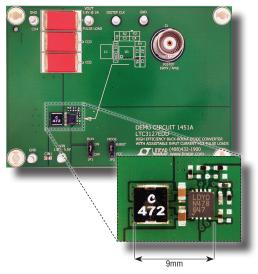
Figure 1. A complete, low profile power converter solution for pulsed load applications
