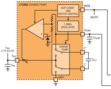
The ideal intermediate step-down regulator would continue to provide power even under cold crank conditions, where the battery voltage can drop below 5V. The LTC3852 does just that—even when its input drops below 5V, its integrated low voltage charge pump produces the necessary 5V drive for the external MOSFETs.
