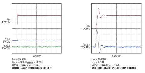
Figure 3. Hot-plug waveform with and without the protection of the LTC4361
