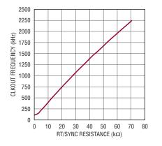
Figure 6. Switching frequency vs RT/SYNC resistance
