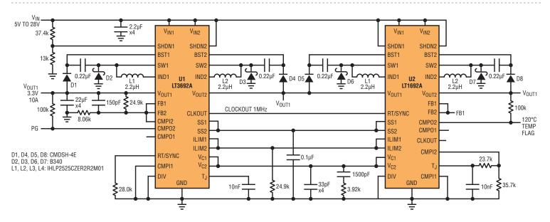
Figure 7. 3.3V, 10A 4-phase converter with UVLO, power good, 120°C junction temperature flag, and minimal input current ripple
