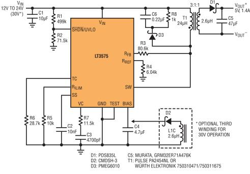
Figure 3. A 12V-24V input, 5V/1.4A output flyback converter
