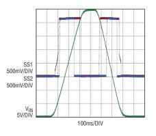
Figure 4. Soft-start voltage during UVLO/OVLO
