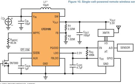
Figure 10. Single-cell-powered remote wireless sensor
