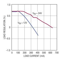
Figure 4. Tight load regulation is achieved from the circuit in Figure 1.
