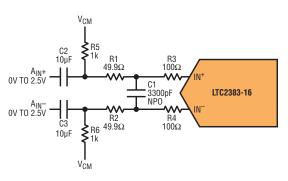
Figure 2. AC-coupled fully differential drive circuit
