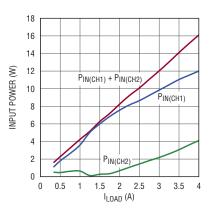
Figure 19. Power draw from two sources for single output
