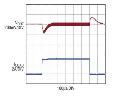
The LTC3113 single inductor buck-boost converter offers a unique combination of features to meet challenging high density power requirements. Internal low resistance switches allow the converter to support an impressive 3A of load current in a tiny 4mm × 5mm package, with peak efficiencies reaching 96%. The internal PWM controller is designed for low noise performance and offers a seamless transition between buck and boost modes.
