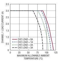
Figure 3. Thermal derating curve for LTC3633 demo circuit (DC1347)
