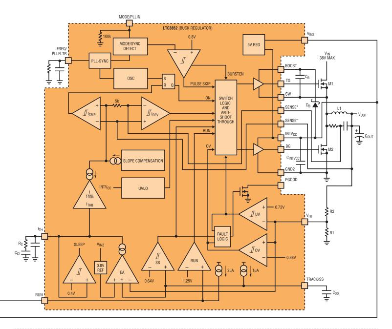
If  $V_{IN}$  falls below 5V, the switching regulator enters dropout operation.  $V_{OUT}$  also falls, but remains high enough for the post-regulator LDOs to continue regulating their output voltages.
