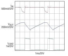
or more of the eight available 577µs time slots. During the remaining time slots, the required load is reduced to less than 100mA, typically. Producing 2A directly from the DC/DC converter would overload the input source, since the pulsed load would draw well in excess of the 500mA guaranteed by USB and PCMCIA. The solution is to use the DC/DC to charge output capacitors to store energy that can be released as needed to satisfy the modem's pulsed-load current draw.
