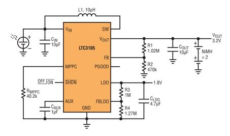
Figure 9. Single-cell photovoltaic NiMH trickle charger
