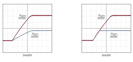
Figure 3. A soft-start capacitor on the TRACK/SS pin can program the ramp time (left), or a resistor divider from one output to the TRACK/SS pin of the other channel can enable the output voltages to track one another during start-up (right).
