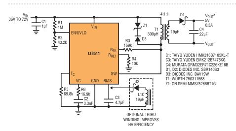
Figure 2. A 48V-to-5V isolated flyback converter using the LT3511 requires remarkably few components
