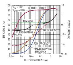
Figure 5. Efficiency and power loss for the three modes of operation. At heavy loads, there is no difference.
