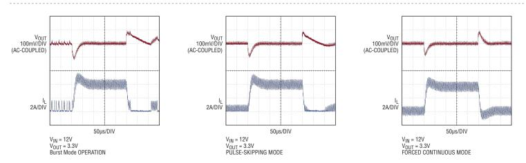
Figure 2. Transient response of Figure 1 for each of the three different modes of operation. At light load, the inductor current is allowed to reverse in forced continuous operation. Burst Mode operation has slightly higher ripple to achieve its much higher efficiency.
