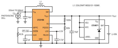
The LTC3105 is a complete single-chip solution for energy harvesting from low cost, single photovoltaic cells.
