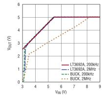
Figure 11. The LT3692A dropout enhancement feature improves dropout performance over a standard buck regulator at high switching frequencies.
