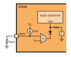
Figure 4. Maximum power point control mechanism
