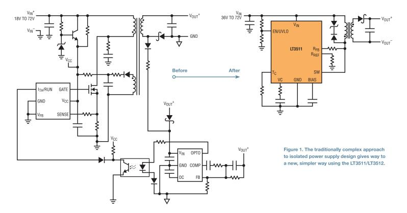
The LT3511/LT3512 infers the isolated output voltage by examining the primary-side flyback pulse waveform. In this manner, neither an opto-isolator nor an extra transformer winding is required to maintain regulation, and the output voltage is easily programmed with two resistors.
