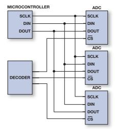
Interfacing several ADCs to a single microcontroller.
