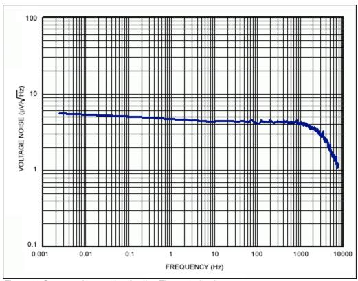
Figure 2. Output voltage noise for the Figure 1 circuit.
