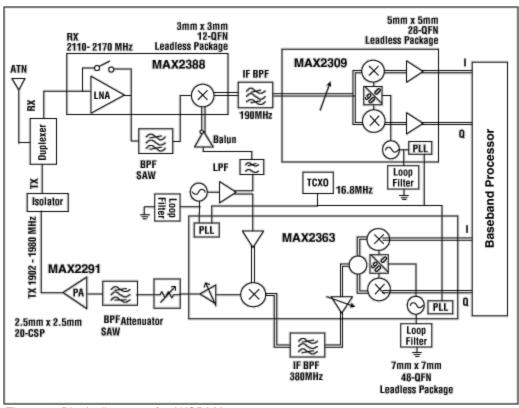
Figure 1. Block diagram of a WCDMA system.
