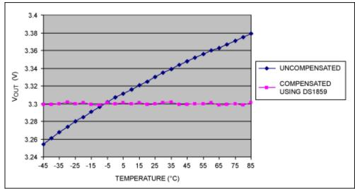
Figure 3. Data plot comparing uncompensated results vs. compensated results.
