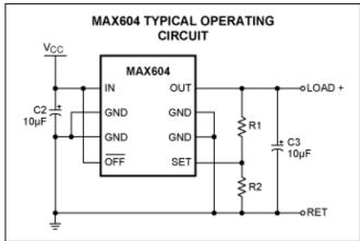
Figure 1. MAX604 shown in adjustable output configuration.
