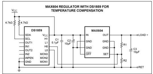
Figure 2. Temperature-compensation circuit for MAX604.
