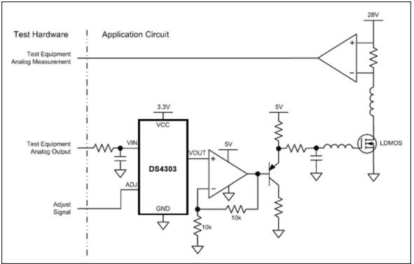
Figure 2. DS4303 LDMOS RF power-amp bias circuit.
