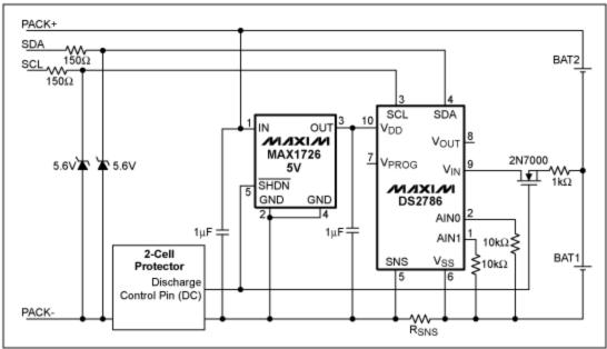
Figure 1. A circuit for using the DS2786 in a 2-cell lithium-ion/polymer pack.
