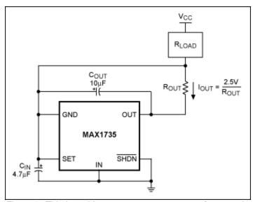
Figure 2. This low-side constant-current source features the MAX1735 and draws  $2.5V/R_{OUT}$  from  $R_{LOAD}$ . This circuit also requires that the voltage for  $R_{OUT}$  between the IN and GND terminals is minimally 2.5V.
