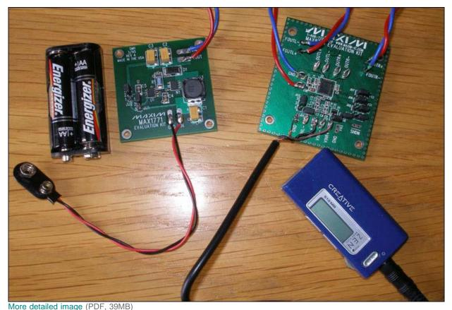
Figure 1. Powered by a switching converter operating from two AA cells, this Class D amplifier (right-hand board) delivers 6W of speaker power for as long as four hours.
