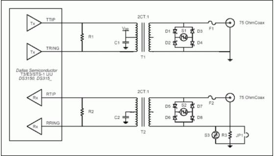
Figure 1. Recommended metallic surge-protection circuit for T3/E3/STS-1.
