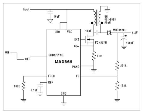
Figure 3. MAX668 SEPIC converter schematic.
