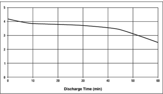
Figure 5. US18650 battery 1C discharge curve.
