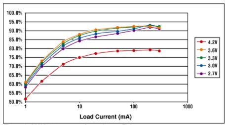
Figure 2. MAX1800 step-up/step-down efficiency.
