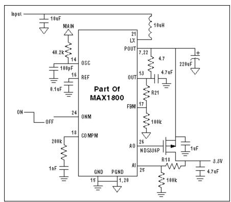
Figure 1. MAX1800 step-up/step-down circuit schematic.
