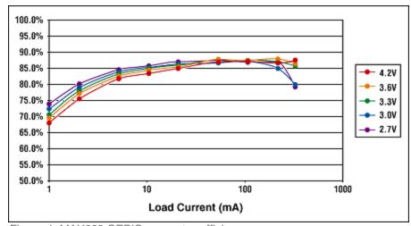
Figure 4. MAX668 SEPIC converter efficiency.
