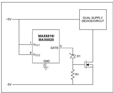
Figure 1. Single-supply, positive/negative voltage sequencer.
