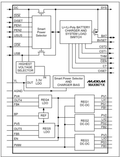
Figure 2. Five independent regulators, plus all battery charging functions and power selection switches, are integrated within the MAX8671X PMIC. Power can be supplied through either an AC adapter or a USB cable.
