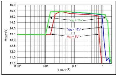
Figure 2. For the circuit in Figure 1, the applied voltage and charging current vary, as shown, during a charge cycle.
