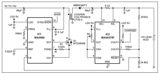
Figure 1. This lead-acid-battery charger applies high voltage (15V) until the battery is charged and then applies 13.4V to maintain a small trickle charge.
