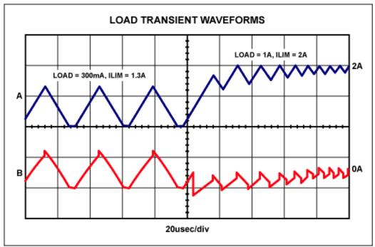
Figure 2. An abrupt change in load current (300mA to 1A) causes changes as shown in the inductor current (top trace, 1A/div) and V<sub>OUT</sub> ripple (ac-coupled bottom trace, 100mV/div).
