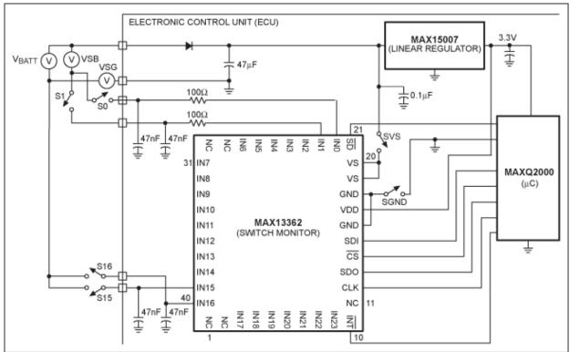
Figure 1. The MAX13362 test circuit.
