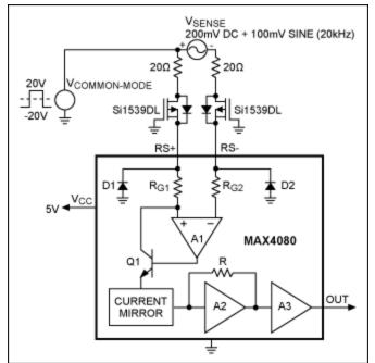
Figure 1. The two p-channel MOSFETs shown protect this high-side current-sense amplifier against negative common-mode voltages.
