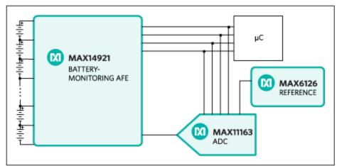
Figure 1. Block diagram of the Maxim solution to optimize the performance of the MAX14921 AFE.
