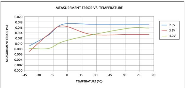
Figure 2. The MAX14921 system measurement error over temperature.
