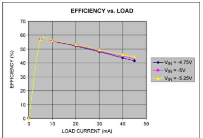
Figure 2. Efficiency vs. load for the Figure 1 circuit at V<sub>IN</sub> levels of -4.75V, -5V, and -5.25V.
