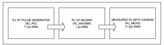
Figure 2. This flowchart illustrates the sequence from which we are able to extrapolate the jitter of the MAX999. Knowing that the HP8082A pulse generator contributes 7.7ps RMS, and that 11.2ps RMS is measured at the CSA8000, we are able to use Equation 1 to extrapolate the MAX999's jitter.
