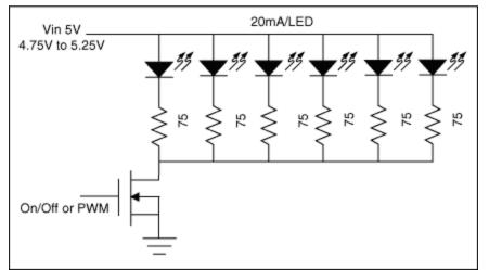
Figure 1. Most applications simply use a fixed bias voltage (5V in this case) and ballast resistors (75 $\Omega$  in this case) to achieve approximate white LED brightness matching.
