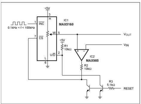
Unlike peak detectors that use a capacitor to hold the output voltage, this design includes a digital potentiometer (IC1) that holds the output level indefinitely, without droop.
