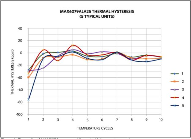
Figure 1. Five units of MAX6079 measured through 10 temperature cycles.
