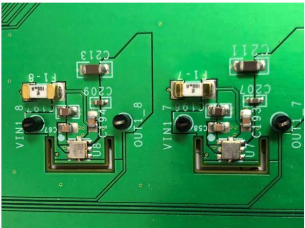
Figure 2. PCB layout with slotting for stress reduction.
