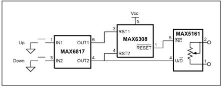
Figure 1. These three ICs form a solid-state potentiometer (EPOT).
