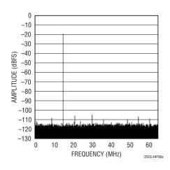
Figure 6a. A 70MHz Low Level Signal with Internal Dither Off. Low Level Tones Are Caused by Small INL Errors in the ADC.
