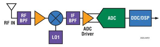
Figure 1. Direct IF to Digital Single Conversion Receiver
