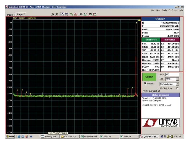
Figure 9. PScope ADC QuickEval Tool-LTC2208 Evaluation
