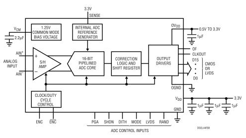
Figure 8. LTC2208 Block Diagram
