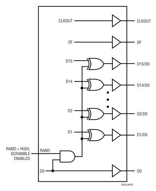
Figure 7. Functional Equivalent of Digital Output Randomizer
