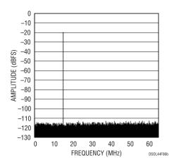
Figure 6b. The Same Conditions with Internal Dither On. Correlated Spurious Tone Energy Has Been Converted to Random Noise
