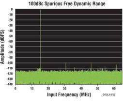
Figure 3. LTC2208 64k FFT F<sub>IN</sub> = 15.2MHz, A<sub>IN</sub> = -1dB, 2.25V<sub>P-P</sub>
