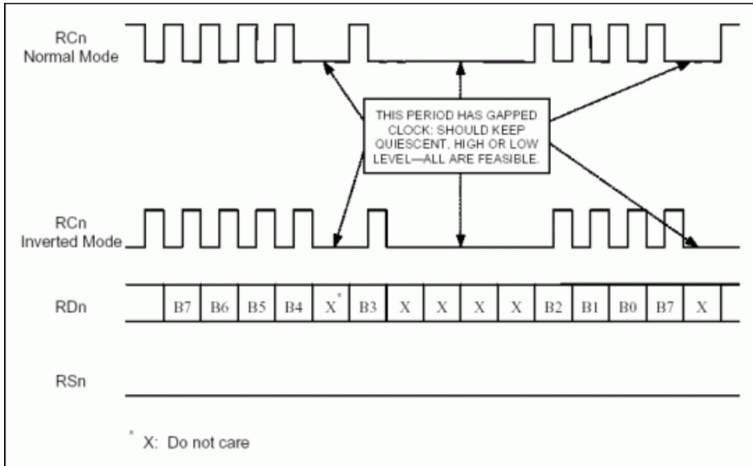
Figure 2. Unchannelized receive link timing with gapped clock.
