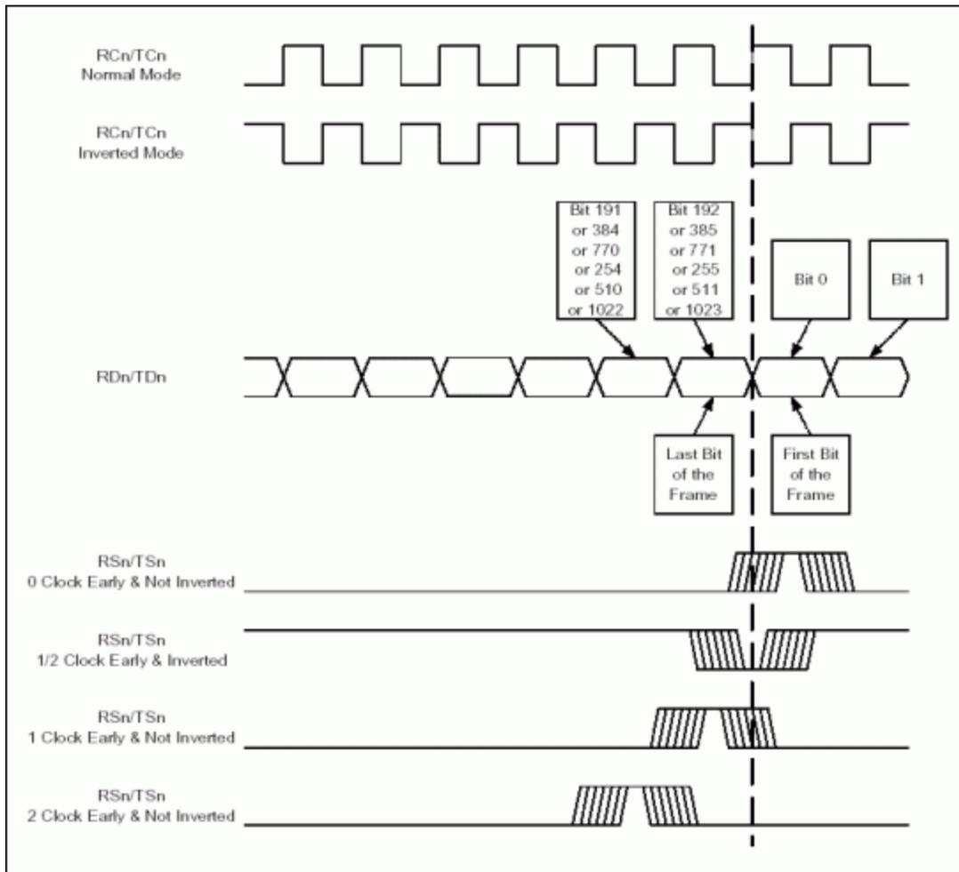
Figure 4. Channelized transmit link timing with normal clock.
