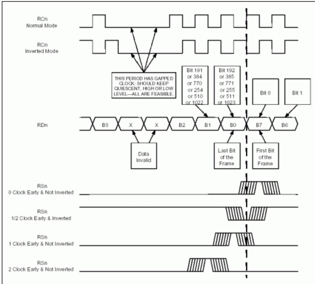
Figure 6. Channelized receive link timing with gapped clock.
