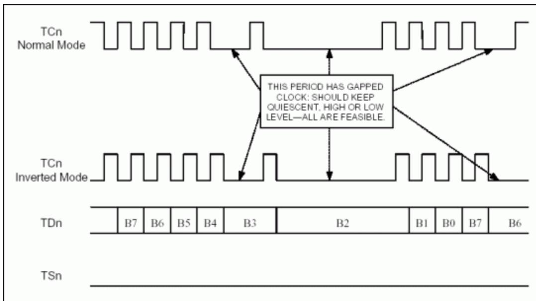
Figure 3. Unchannelized transmit link timing with gapped clock.
