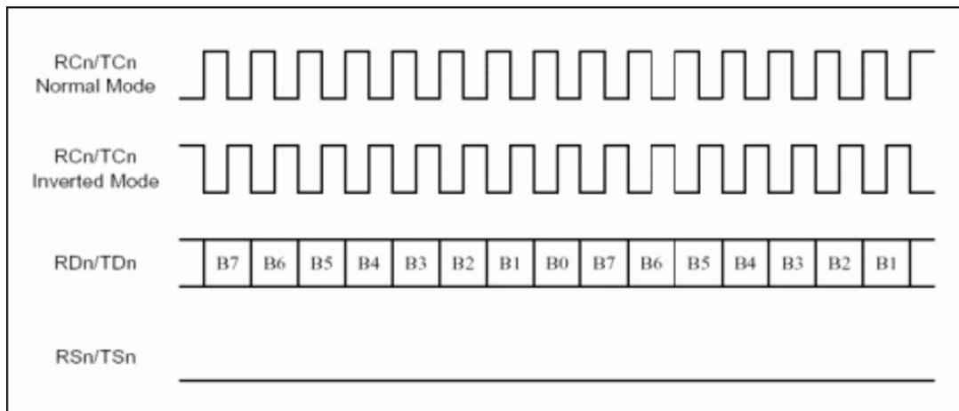
Figure 1. Unchannelized link timing with normal clock.
