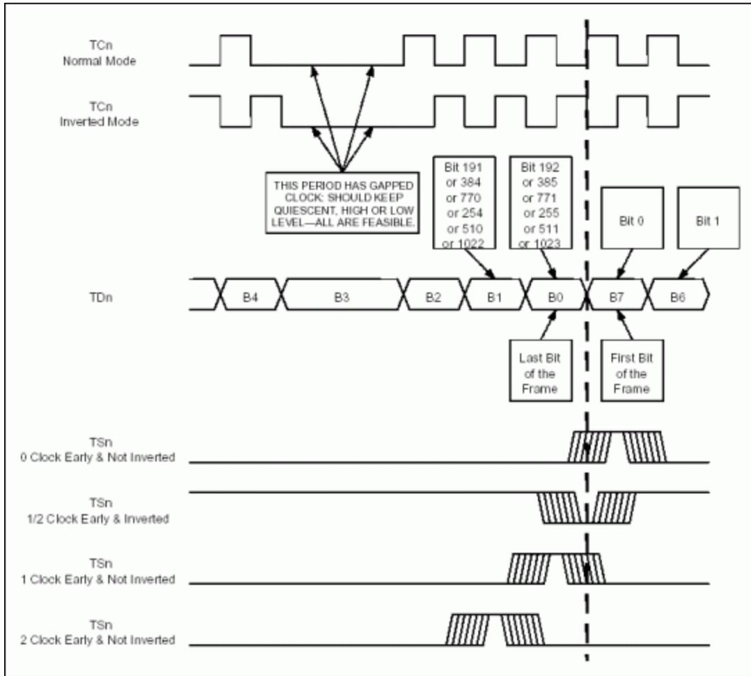
Figure 7. Channelized transmit link timing with gapped clock.
