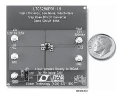
Figure 1. The LTC3250 Is Available in a Tiny 6-Pin ThinSOT Package Making it Possible to Fit a Complete Converter in Less Than 0.04in<sup>2</sup>
