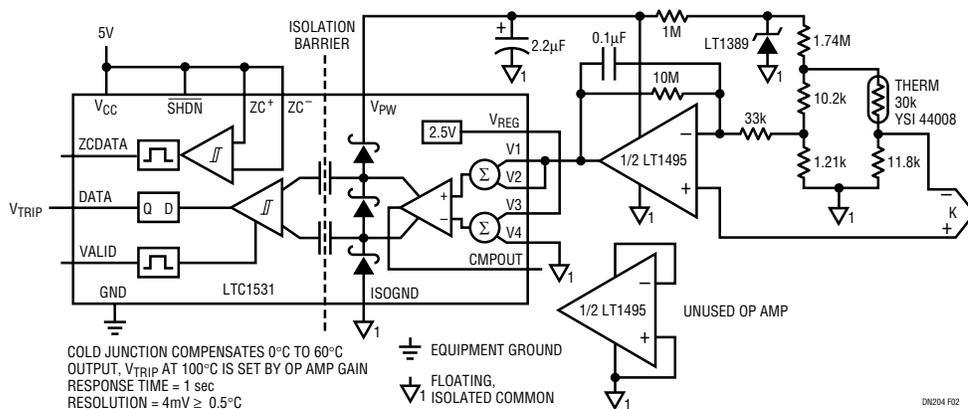
Figure 2. Overtemperature Detect
