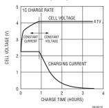
Figure 1. Typical Lithium-Ion Charge Characteristics
