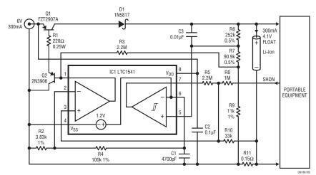
Figure 2. Lithium-Ion Battery Charger
