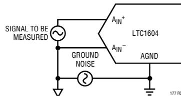
**Figure 5. The LTC1604's Differential Inputs Reject Common Mode Noise by Measuring Differentially**
