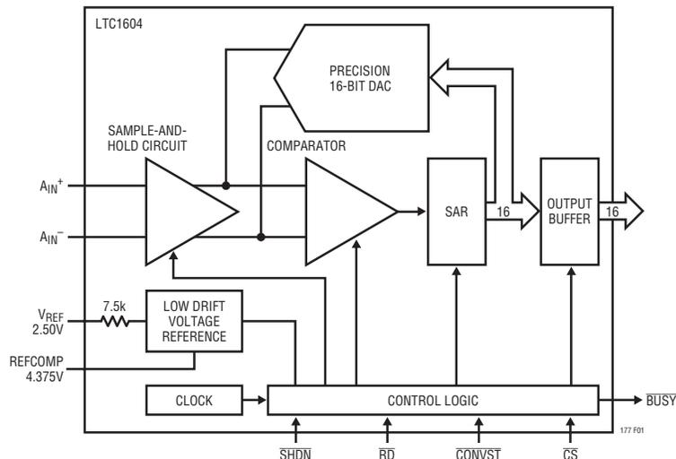
Figure 1. The 333ksps, 16-Bit ADC Features a True Differential S/H with Excellent Bandwidth and CMRR
