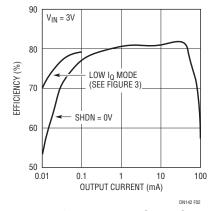
Figure 2. Efficiency vs Output Current
