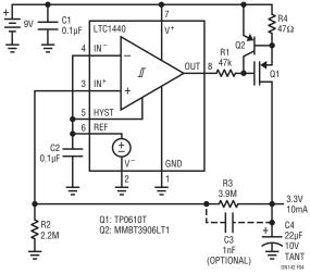
Figure 5. Micropower LDO Regulator
