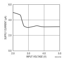
Figure 4. No-Load I<sub>CC</sub> vs Input Voltage for Low I<sub>O</sub> Mode
