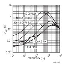
Figure 5. LT1118-2.5 Output Impedance vs Frequency
