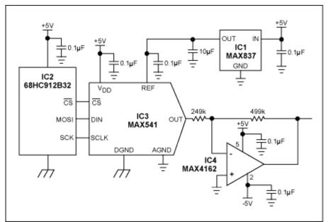
Figure 1. This compact circuit enables microcontroller IC2 to generate a variable negative voltage.
