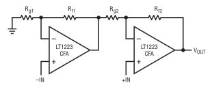
TRIM  $R_{g2}$ FOR GAIN, THEN TRIM  $R_{g1}$  FOR CMRR. VOLTAGE GAIN, G, IS  $V_{OLT}$  DIVIDED BY DIFFERENCE BETWEEN +IN AND -IN.
