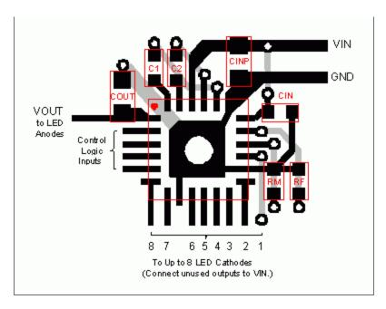
Observe the following guidelines when laying out PCB artwork for the MAX1576 white-LED charge pump:
