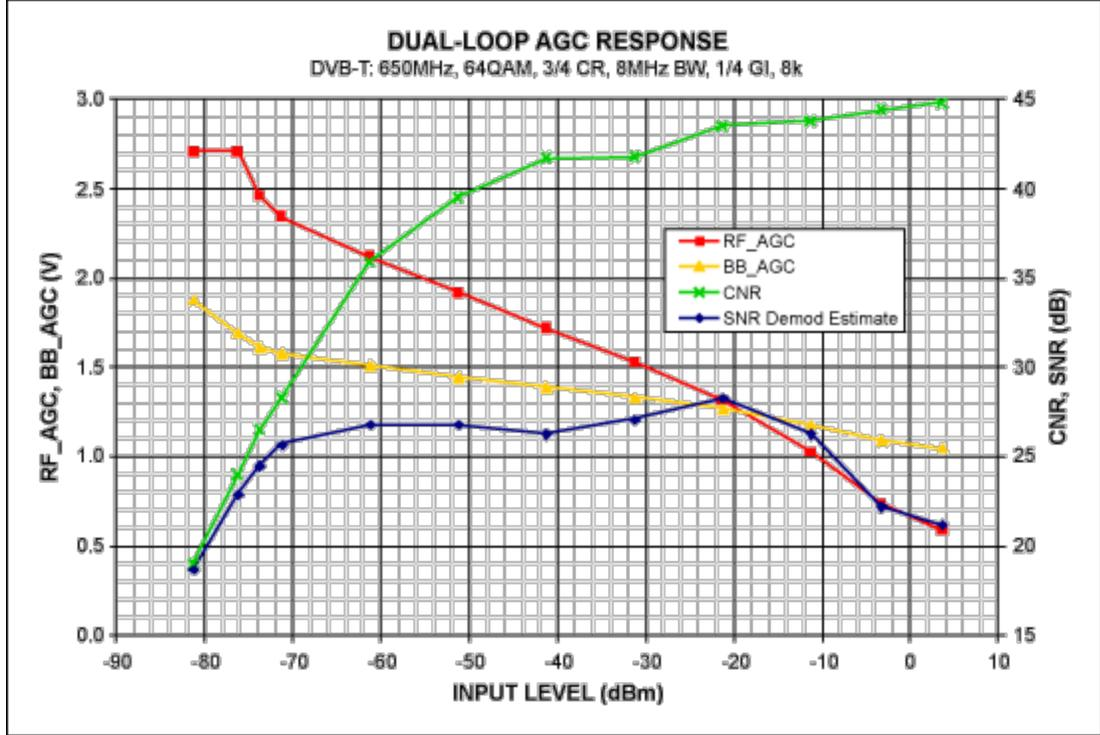
Figure 7. Dual-loop AGC response with wanted signal only.
