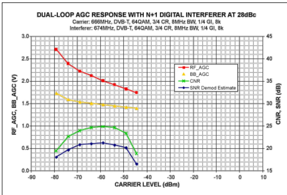
Figure 8. Dual-loop AGC response with a N+1 digital interferer at 28dBc.
