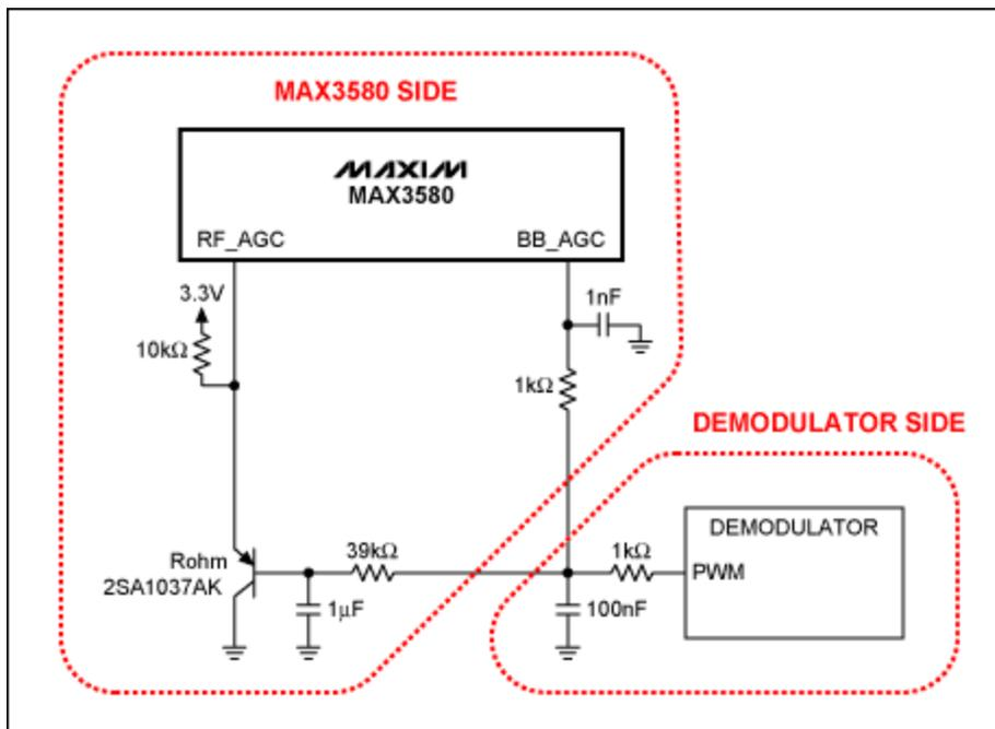
Figure 10. Single-loop AGC schematic.
