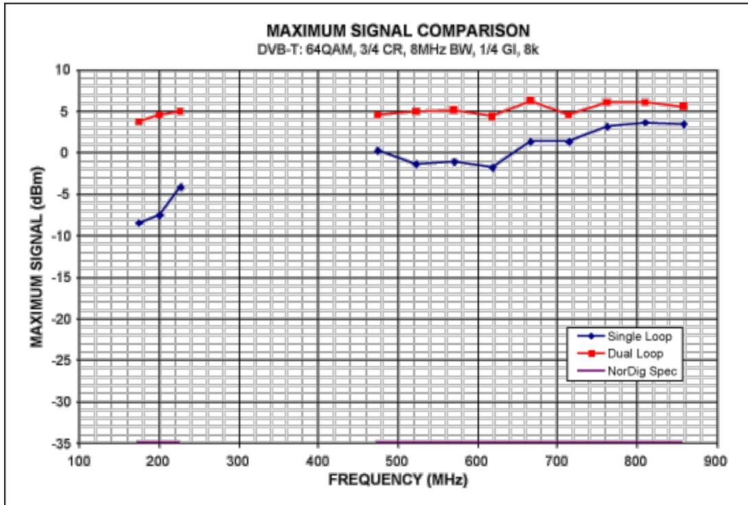
Figure 2. Maximum signal comparison between dual-loop and single-loop AGC control.
