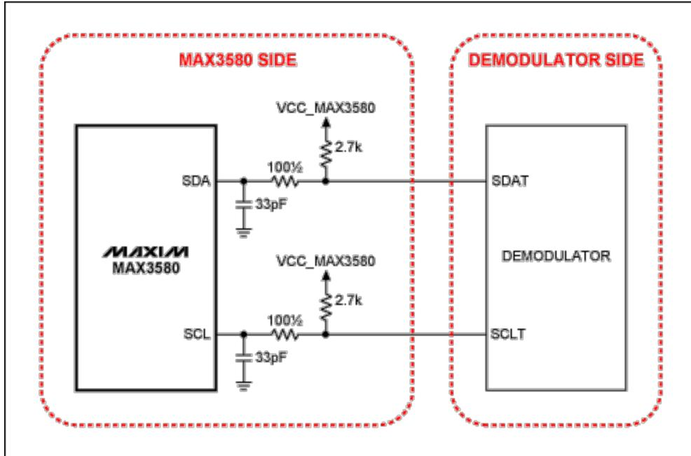
Figure 13. Recommended I<sup>2</sup>C line filtering.
