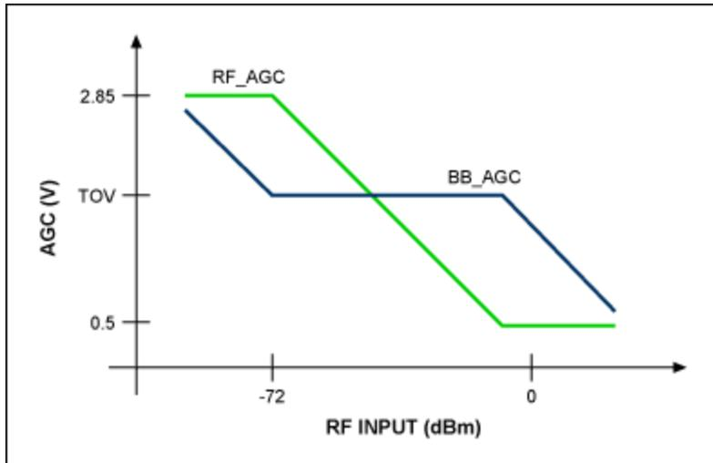
Figure 9. Alternate dual-loop gain control.
