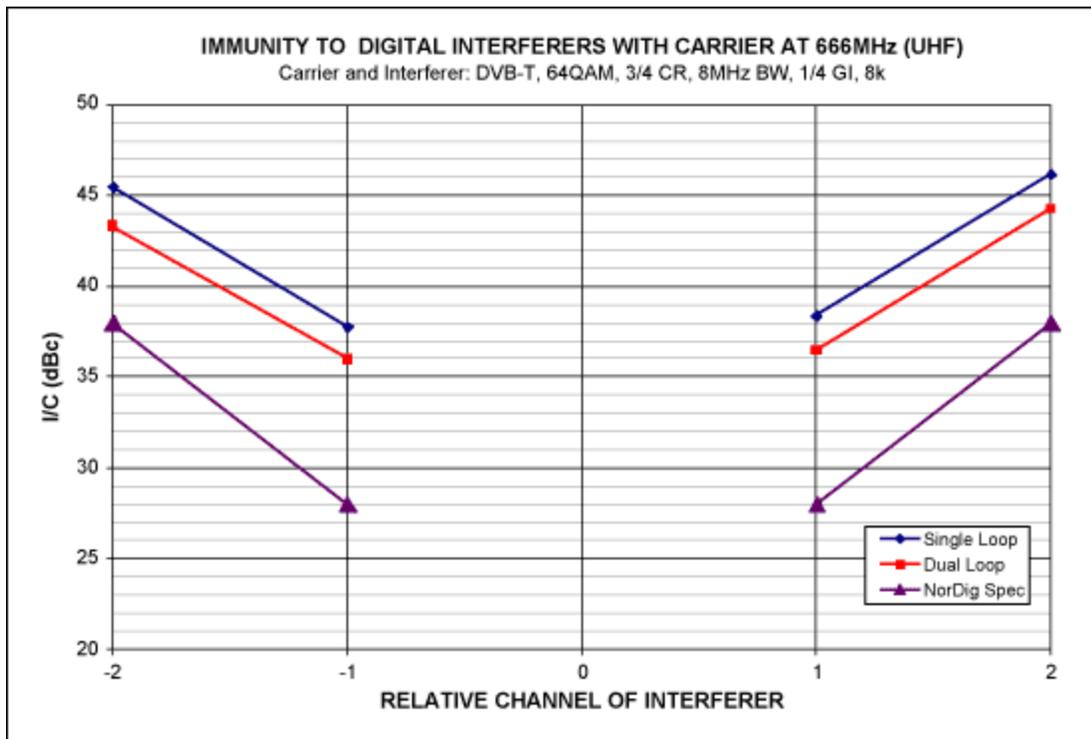
Figure 4. Digital I/C comparison between dual-loop and single-loop AGC control at UHF.
