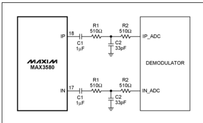
Figure 12. Recommended I channel interface (duplicate for Q channel).
