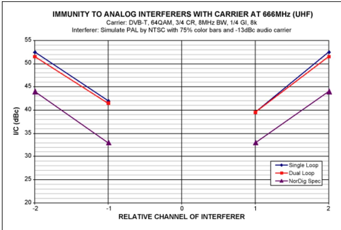
Figure 5. Analog I/C comparison between dual-loop and single-loop AGC control.
