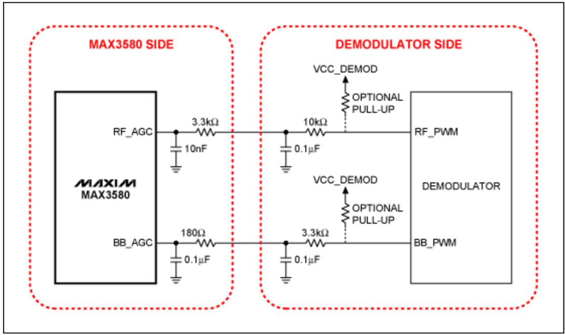
Figure 6. Dual-loop AGC schematic.
