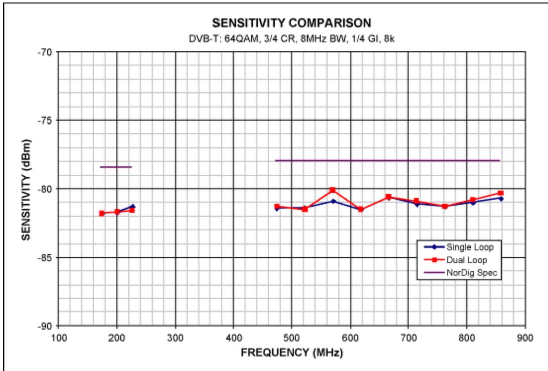
Figure 1. Sensitivity comparison between dual-loop and single-loop AGC control.
