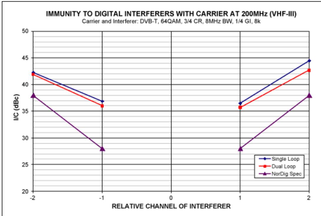
Figure 3. Digital Interference-to-Carrier (I/C) comparison between dual-loop and single-loop AGC control at VHF-III.
