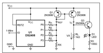
Figure 1. This 4-bit DAC is controlled by a 1-Wire interface. (DS2408 outputs P4 to P7 are not used.)
