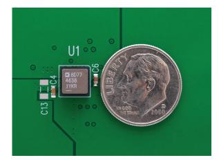
Figure 2. Tiny 15 A dc-to-dc  $\mu$ Module regulator solution using the LTM4638 on a DC2665A-B demonstration board. Input and output capacitors are shown here a few ceramic capacitors and a resistor are on the back of the board.
