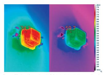
Figure 4. Effective airflow cooling with CoP design is clear in this comparison of 0 LFM and 200 LFM airflow on thermal performance of the LTM4638 at 12 V input, 1 V output at 15 A.
