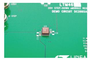
Figure 6. The LTM4626 on a DC2665A-A demonstration board.
