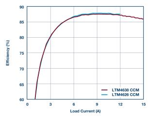
Figure 5. Efficiency of the LTM4626 and LTM4638 with 12 V input, 1 V output, operating at 600 kHz.
