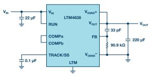
Figure 3. The LTM4638 12 V input, 1 V output, 600 kHz simplified schematic using only ceramic capacitors and minimal components. Floating pins are not displayed.
