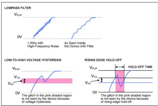
Figure 1. New 1-Wire front-end features.
