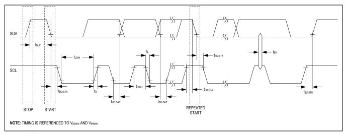
Figure 1. I<sup>2</sup>C Timing Diagram
