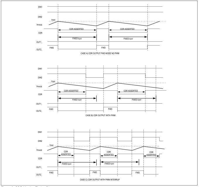
Figure 2. CDR Monitor Timing Diagram
