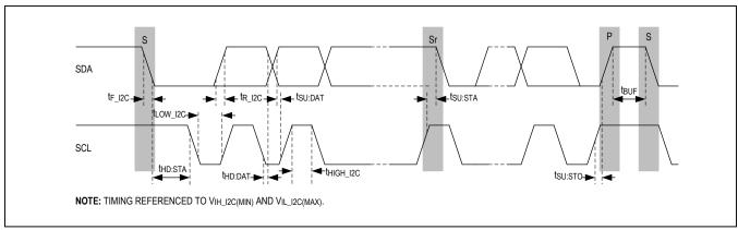
Figure 7. I<sup>2</sup>C Bus Controller Timing Diagram
