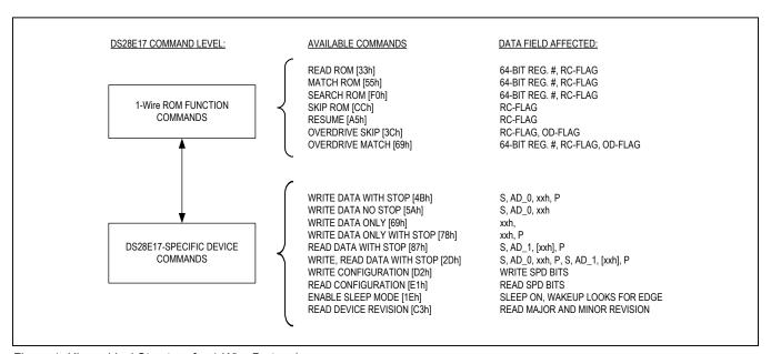
Figure 1. Hierarchical Structure for 1-Wire Protocol
