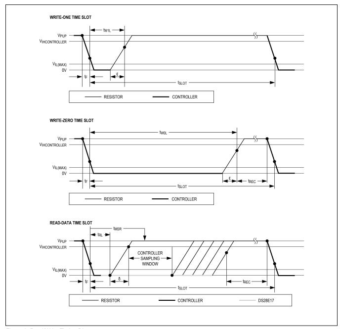
Figure 6. Read/Write Timing Diagrams
