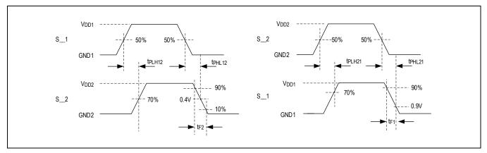
Figure 2. Timing Parameter Definition
