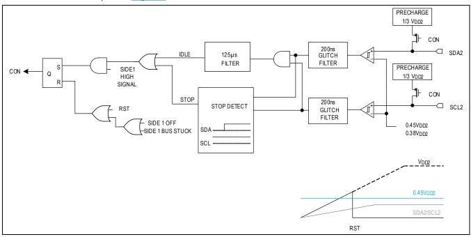
Figure 7. Bus Connection Logic
