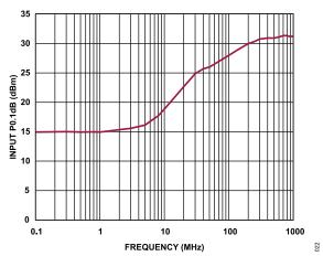
Figure 22. Input P0.1dB vs. Frequency, Low Frequency Detail
