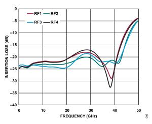
Figure 9. Insertion Loss for RFC when RFx Selected vs. Frequency
