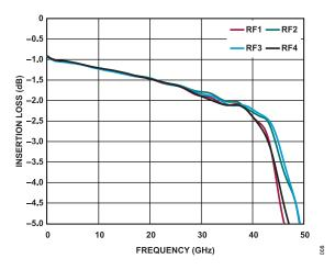
Figure 8. Insertion Loss for RFC to RFx Selected vs. Frequency
