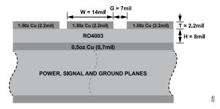
Figure 25. Example PCB Stackup
