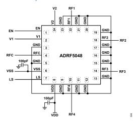
Figure 24. Recommended Schematic
