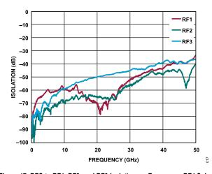
Figure 17. RFC to RF1, RF2, and RF3 Isolation vs. Frequency, RF4 Selected
