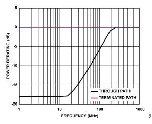
Figure 2. Power Derating vs. Frequency, Low Frequency Detail, T<sub>CASE</sub> = 85°C
