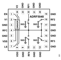
Figure 1. Functional Block Diagram
