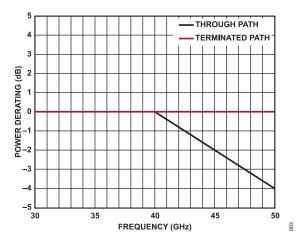
Figure 3. Power Derating vs. Frequency, High Frequency Detail, T<sub>CASE</sub> = 85°C
