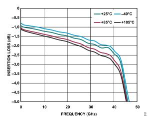
Figure 11. Insertion Loss for RFC to RF1 vs. Frequency over Temperature
