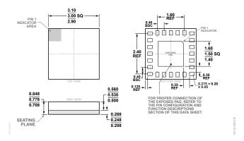
Figure 28. 24-Terminal Land Grid Array [LGA] (CC-24-14) Dimensions shown in millimeters
