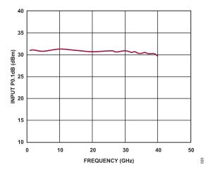
Figure 20. Input P0.1dB vs. Frequency
