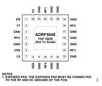
Figure 4. Pin Configuration
