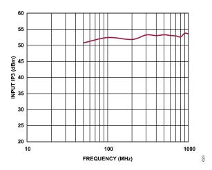
Figure 23. Input IP3 vs. Frequency, Low Frequency Detail
