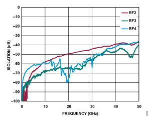
Figure 10. RFC to RF2, RF3, and RF4 Isolation vs. Frequency, RF1 Selected
