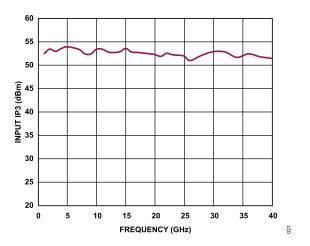
Figure 21. Input IP3 vs. Frequency
