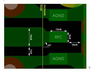
Figure 27. Recommended RFx Pin Transitions
