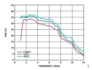
Figure 24. PAE vs. Frequency, 1 GHz to 12 GHz, for Various Temperatures,  $V_{DD}$  = 5 V,  $I_{DQ}$  = 55 mA
