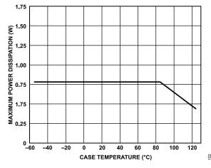
Figure 2. Maximum Power Dissipation vs. Case Temperature
