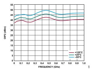
Figure 26. OIP2 vs. Frequency, 0.01 GHz to 1.0 GHz, for Various Temperatures,  $V_{DD} = 5 \text{ V}$ ,  $I_{DQ} = 55 \text{ mA}$
