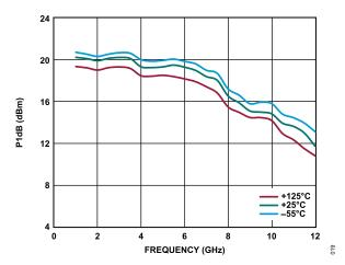
Figure 19. P1dB vs. Frequency, 1 GHz to 12 GHz, for Various Temperatures,  $V_{DD}$  = 5 V,  $I_{DQ}$  = 55 mA
