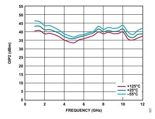
Figure 27. OIP2 vs. Frequency, 1 GHz to 12 GHz, for Various Temperatures,  $V_{DD}$  = 5 V,  $I_{DQ}$  = 55 mA
