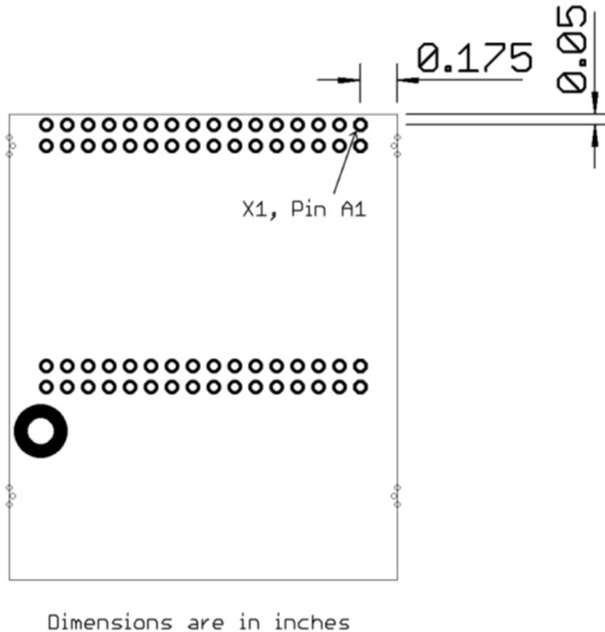
Figure 5 - Location of X1 connector and Pin A1
