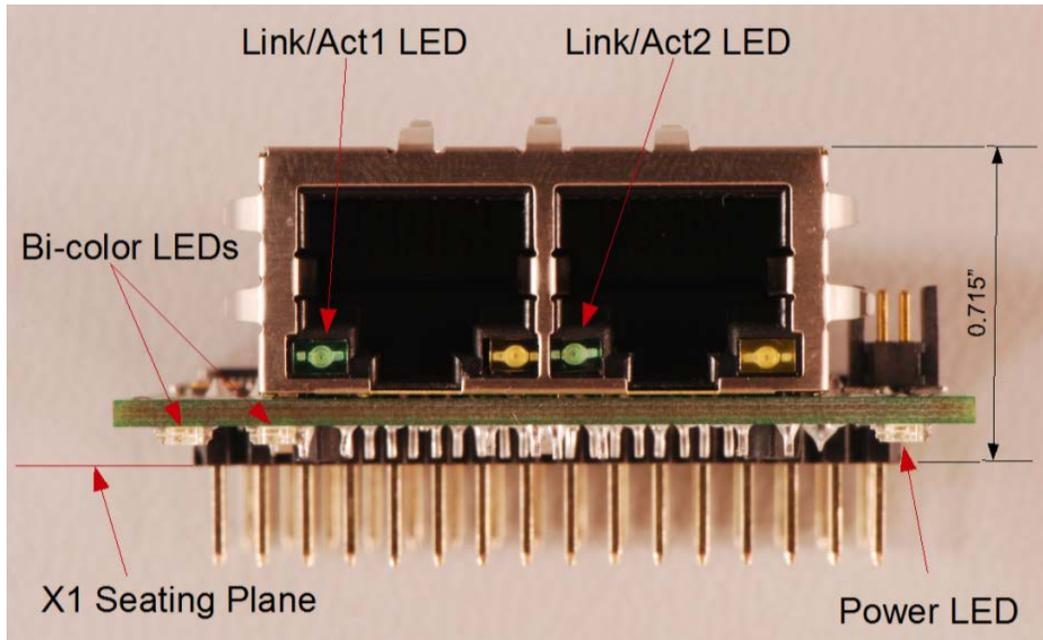
Figure 3 - Dimensions of the Network Interface Module (Cross-section)
