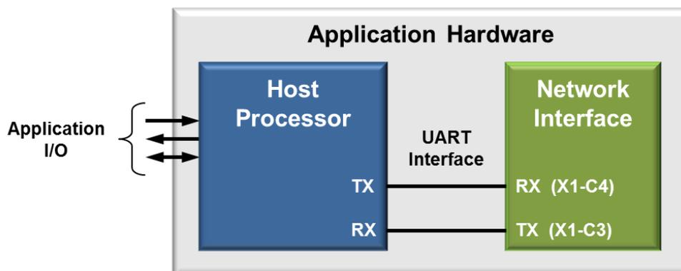
Figure 7 – UART Host Interface Connection for Module
