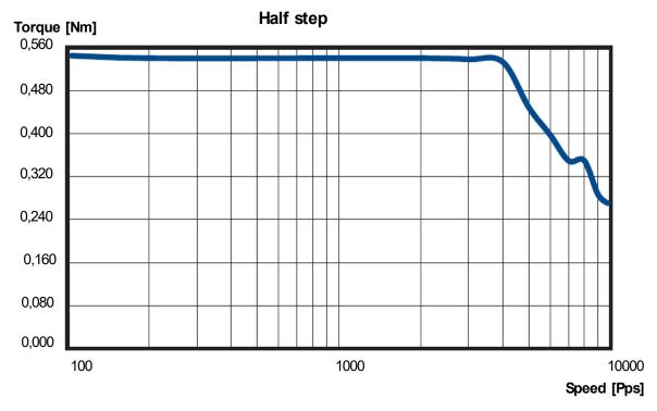
Figure 5.1: QSH5718-41-28-055 speed vs. torque characteristics
